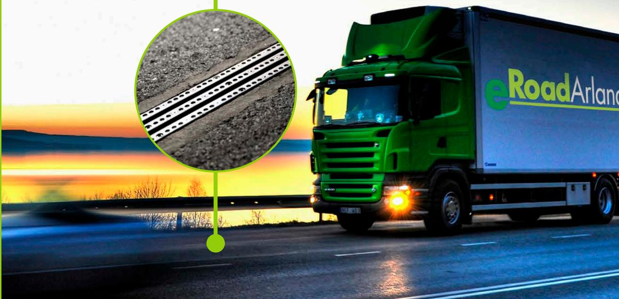
Electrified roads with conductive feeding from below works for all types of transports, both cars and larger vehicles such as buses and trucks. Energy is transferred from the rail in the road to the vehicle using a movable arm. As long as the vehicle is above the rails, the contact is in the down position. When overtaking another vehicle it's automatically lifted up.
